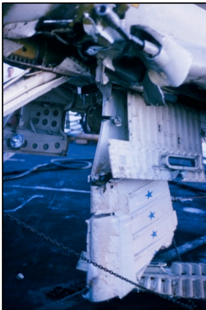
Fig. 1 Close-up of stabilizer sticking into the fuel tank of Lt. Ilg's A4-C Skyhawk after it made an emergency landing on Midway. Read story below to learn how it got there. Also see Fig. 2 (below) of his Skyhawk.
