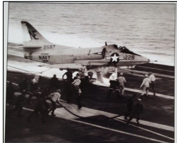
Fig. 2 Lt. Ilg's A4 on Midway's flight deck showing the vertical stabilizer of the other A4 embedded in the underside of his plane (look directly below the intake). This photo was probably taken from Pri-Fly.
