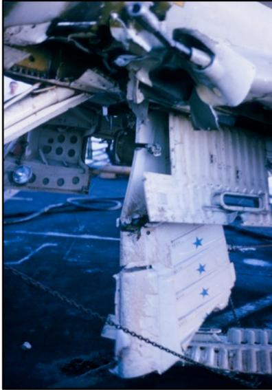
**Fig. 1** Close-up of stabilizer sticking into the fuel tank of Lt. Ilg’s A4-C Skyhawk after it made an emergency landing on Midway. Also see Fig. 2 (below) of his Skyhawk.
