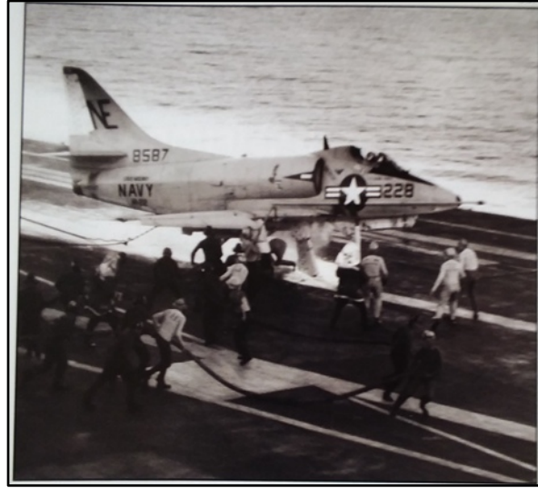
Fig. 2 Lt. Ilg's A4 on Midway's flight deck showing the vertical stabilizer of the other A4 embedded in the underside of his plane (look directly below the intake). This photo was probably taken from Pri-Fly.
